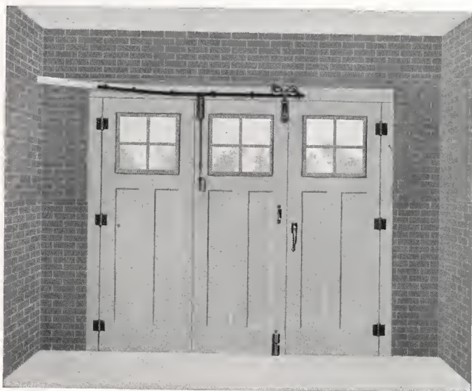
Inside view, showing doors closed. As they open inward, snow and ice cannot interfere. Doors swing into jamb against stops. (For description, see page 52.)
